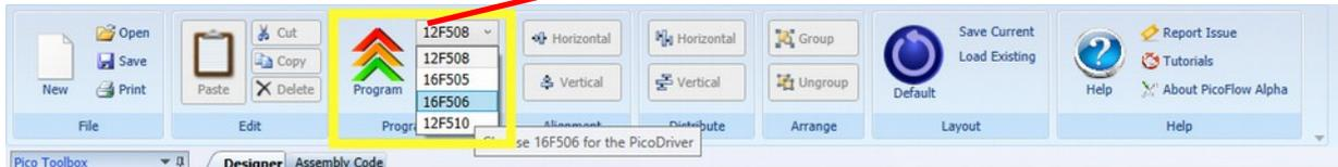
The PicoPi uses a PIC called the PIC16F506<sup>(1)</sup>. This device can be selected in PicoFlow Alpha on the Programming Panel of the Ribbon Bar.
