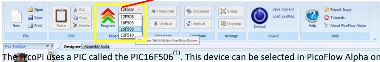
The PicoPi uses a PIC called the PIC16F506<sup>(1)</sup>. This device can be selected in PicoFlow Alpha on the Programming Panel of the Ribbon Bar.
