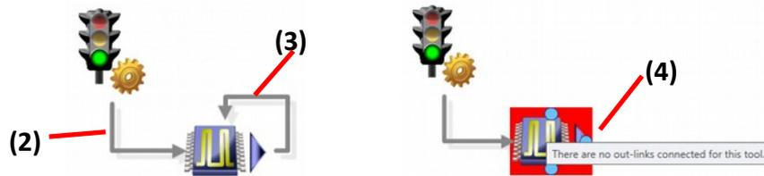
The Output Tool must be linked up<sup>(2)</sup> from the Start Tool and at the end the links must loop<sup>(3)</sup> back to the Output Tool. If you don't link it up at the end, then you will receive an error<sup>(4)</sup>.
