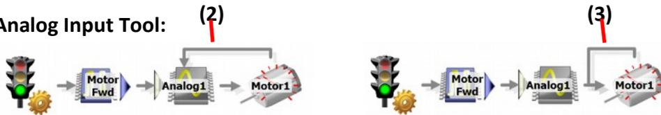
The Analog Input Tool must be linked up in a loop<sup>(2)</sup> so the value updates regularly. **Warning:** Incorrect Linking with the Analog Tool out of the loop<sup>(3)</sup> will not vary the speed of the motor.
