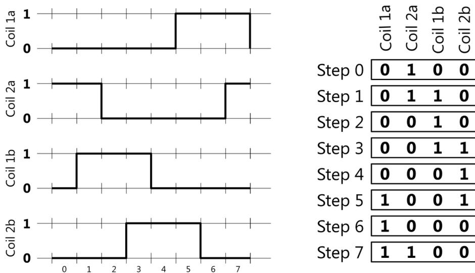
**Stepper Motor 8 Step Sequence - Graph and Binary Table**
